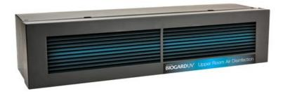
Each of these devices utilizes a mercury-vapor lamp that emits invisible ultraviolet light at a wavelength of 254 nanometers (nm). An internal aluminum reflector and louvers on the front surface cause the emitted UVC light to fan-out horizontally while limiting the vertical projection to a relatively thin layer eight to ten feet above the floor. As the UV field is well above-head, the room remains safe for occupancy while the air is continuously disinfected.
